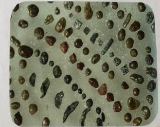
Photograph shows galena, minium and native lead (stereomicroscope x200).
