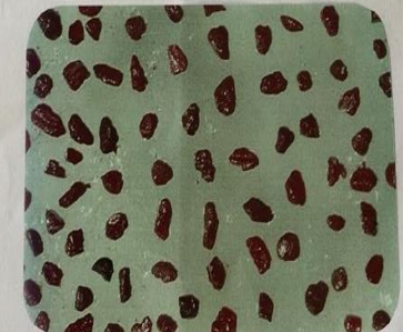
Photograph shows cinnabar (stereomicroscope x200).
