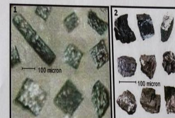
Fig. (86): Stereomicrographs showing galena grains.
